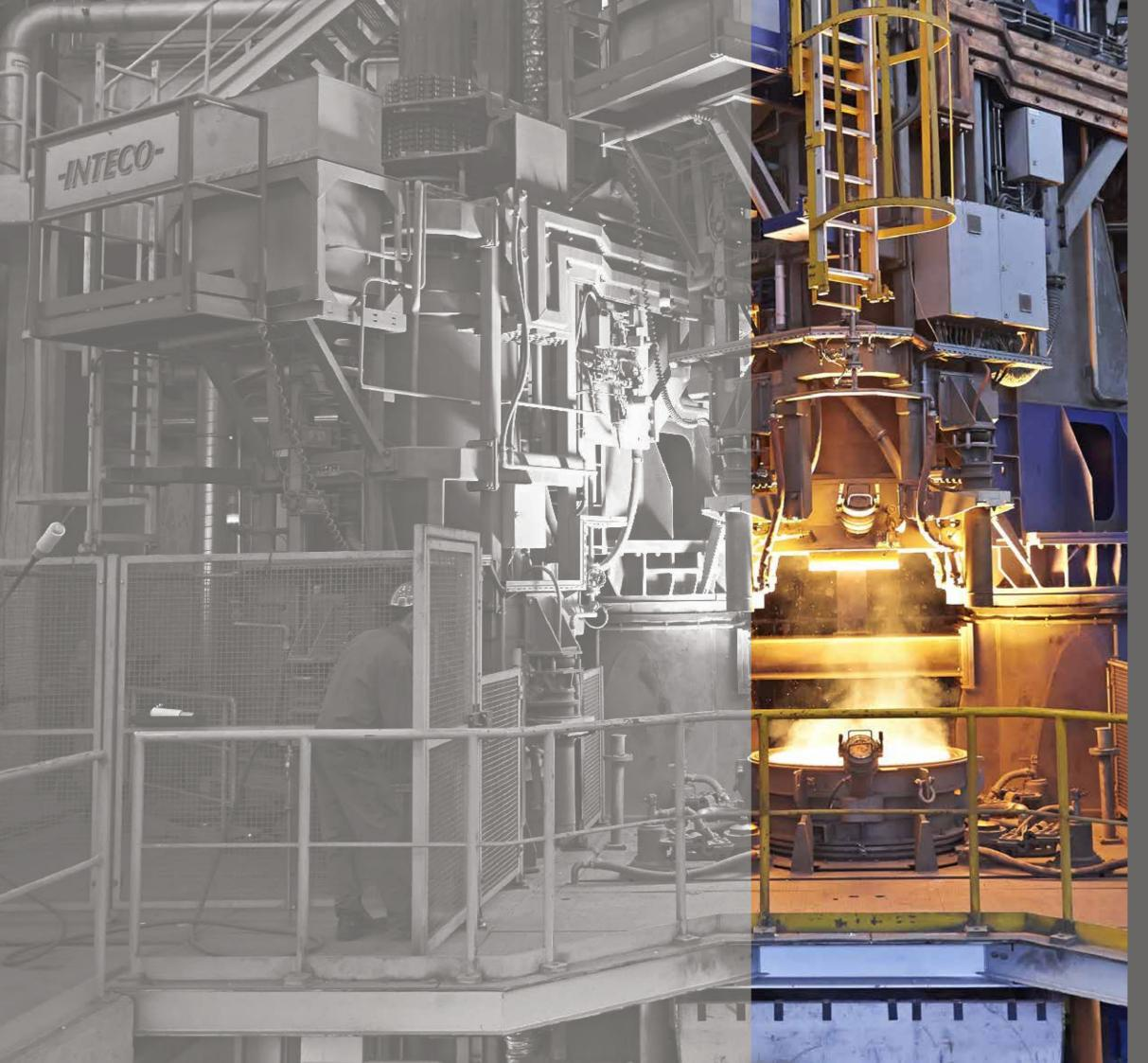
THE ELECTROSLAG REMELTING PLANT features two large 36 and 50 ton ESR furnaces and a smaller one of 3 ton. Via ESR method we can produce extra clean tool steels to ensure the maximium perfomance of the tool. Based on ESR remelting, we are also developing customized tool steel grades to meet requirements for even the most demanding tooling applications.
