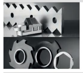
SIKNIVES for shredding are manufactured from the new generation of steel alloys with different hardening processes (through-hardened, casehardened, nitrided, etc.) and heat treated in vacuum to maximise blade performance.
